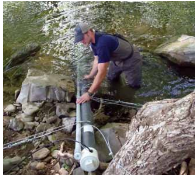
Matt Shank of the SRBC installs a water quality sonde in a PVC pipe to endure winter and summer conditions. (Photo: Heather Hardeman)
