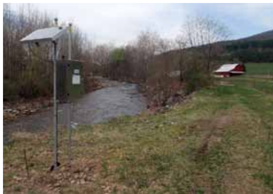
A network of 50 remote water quality monitoring stations is designed to cover a wide range of locations and detect frac fluid spills. (Photo: Andrew Gavin)
